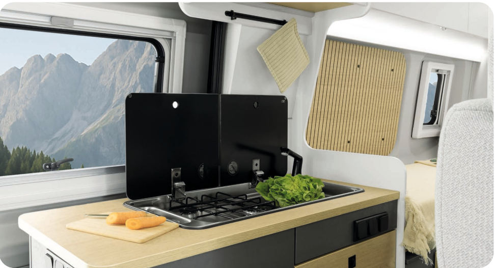
Integrated sink and 2-burner stove with piezo ignition and covers.
